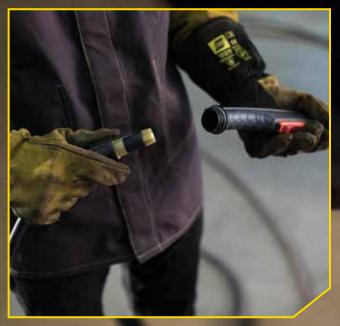
stands for quick disconnect, which gives you the option of replacing only what you need to replace – the torch or the lead – and that saves you money in the long run.
