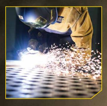
**Long arc stretch** – When you are in an odd position or trying to hit a corner, Cutmaster 60i's extra-long arc will stretch to keep constant contact with the workpiece.
